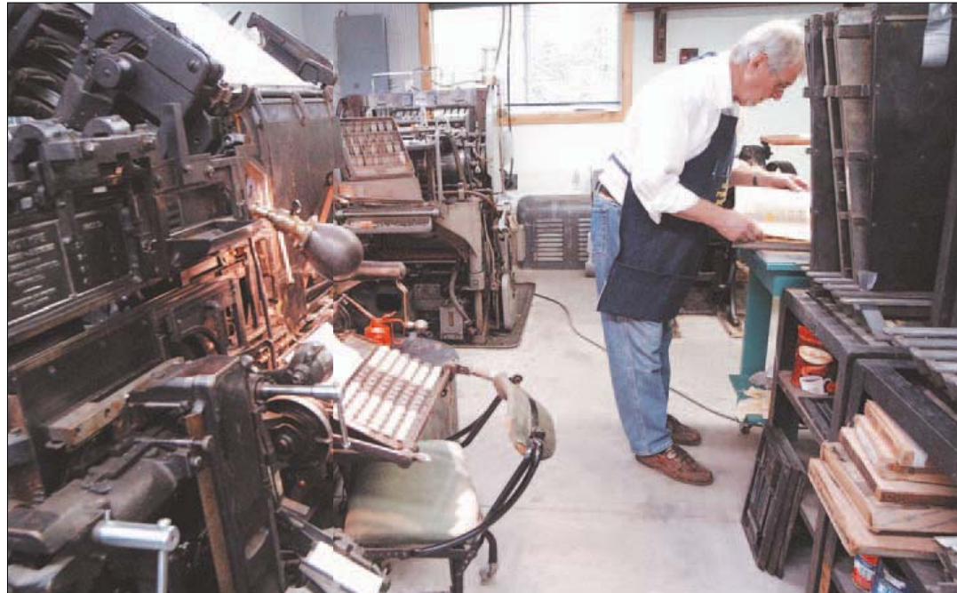
Davis's collection of presses inside his shop near Bala includes a classic Linotype (left) which he uses to set type. He uses a Chandler letterpress to create his sought-after wedding invitations that give words a striking 3-D appearance.
